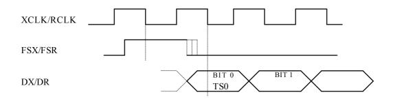
Timings diagram of 29C94 PCM line (T1 - slave/master mode)
