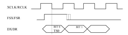
Timing diagram of 29C96 PCM line (E1-T1 mode)
